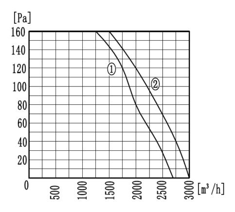
Curve 1: 50HZ Curve 2: 60HZ
